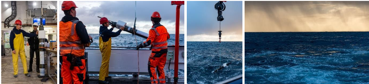
A buoy from the international ARGO ocean monitoring program is deployed during MSM111. The instrument is first switched on with a magnet and then released overboard with a crane before it disappears into the ocean waves. Photos: Volker Diekamp.
