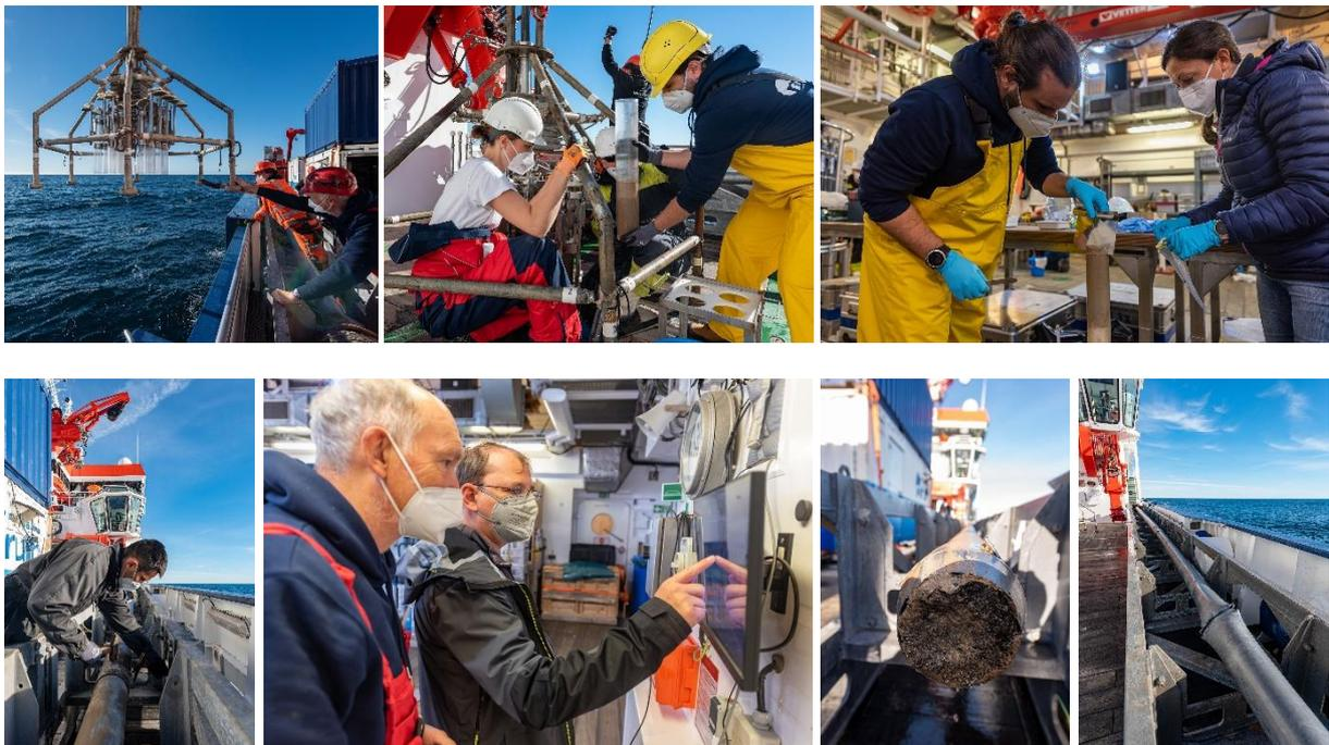
*Top left: the multicorer is lowered to the seafloor, the recovered short cores are separated from the instrument on deck (center) and processed in the laboratory (right). Bottom left: the gravity corer is prepared on deck, deployment is monitored in the geolab (center). The 18 m gravity corer accidentally bent in the middle of the tube back on board with volcanic rocks in the core catcher (left). All photos: Volker Diekamp.*
