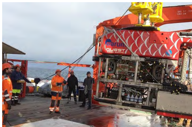
Figure 2: Deploying the MARUM ROV QUEST from the aft deck of the RV MARIA S-MERIAN in the early morning with changing weather conditions (© Gerhard Bohmann).
