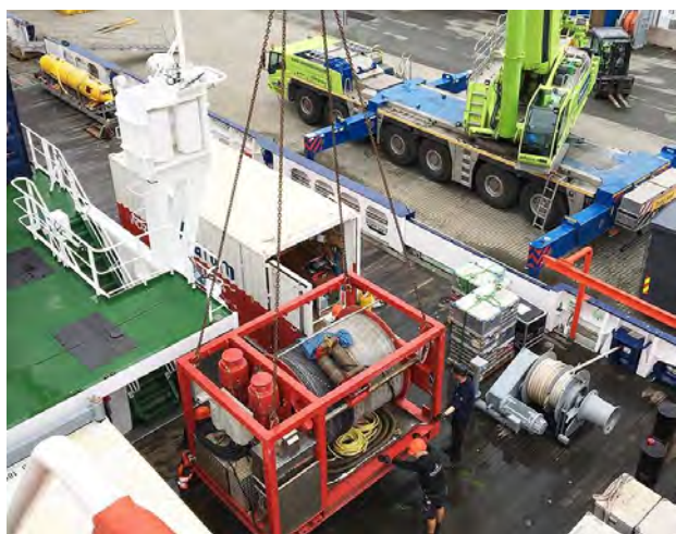
Figure 1: At Pier 24 in the port of Breivika/Tromsø, a special crane has hoisted the 18 t ROV winch onto the aft deck of RV MARIA S. MERIAN (© Gerhard Bohrmann).
