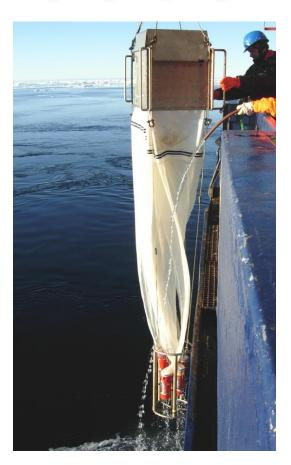
Fig. 3: Deployment of the multinet to catch zooplankton organisms at discrete depths in the water column.
