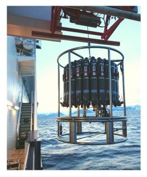
Fig. 1: Deployment of the CTD / Rosette Water Sampler off Spitsbergen.
