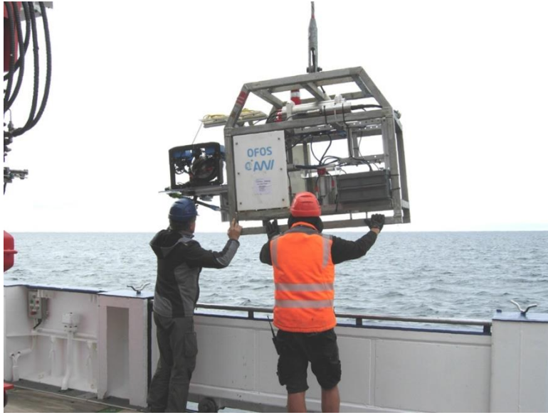
Fig. 3: Deployment of the towed photo/video system OFOS (Ocean Floor Observation System) for seafloor mapping and to assess distribution patterns of larger benthic organisms.
