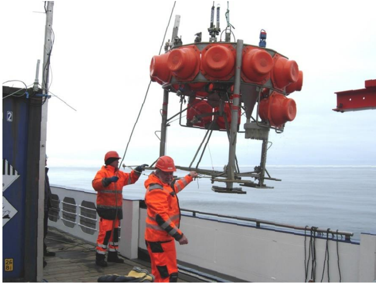
Fig. 1: Recovery of the Long-Term Bottom-Lander after one year at the central HAUSGARTEN site
