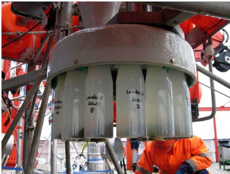
Fig. 2: Carousel of sampling bottles of the sediment trap to assess the flux of particulate matter to the deep seafloor.
