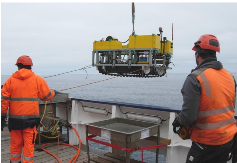
Fig. 3: First test trials of the new Benthic Crawler of the AWI deep-sea group to assess remineralisation rates at the deep seafloor.
