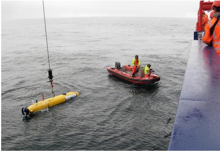
Fig. 1: Recovery of the Autonomous Underwater Vehicle (AUV) „PAUL“ after mapping the seafloor at the LTER Observatory HAUSGARTEN.
