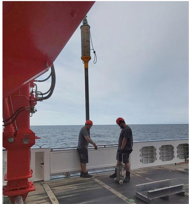
*Fig. 5: Sampling with the gravity corer. (Photo: Sebastian Hölz)*
