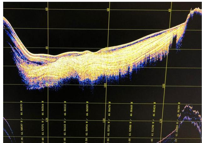
Fig. 4: Sediment-filled depression imaged by the sediment echo sounder (Parasound).
