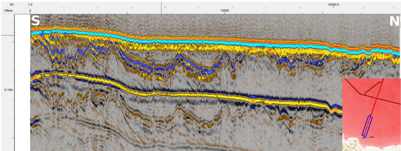
Fig. 3: Seismic section along the main profile directly north of the PEI. Due to the shallow water depth (<50m), the sea floor is visible as a strong reflector even for very short periods of time. A heavily structured layer lies directly underneath. The deeper areas of the section are heavily influenced by multiples due to the shallow water depth.
