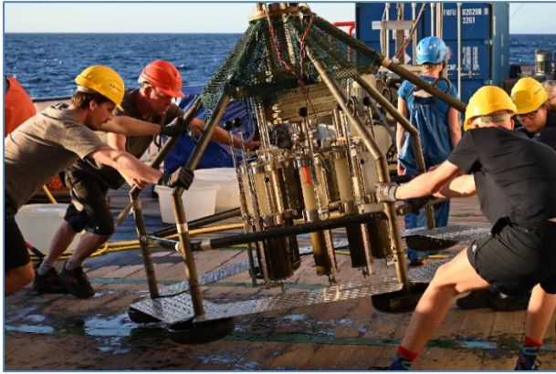
Left picture: Michael Kossack, Andreas Wolff, Simon Pörrmann and Antonia Witzleb (from left) hauling in the multicorer with filled core tubes.
