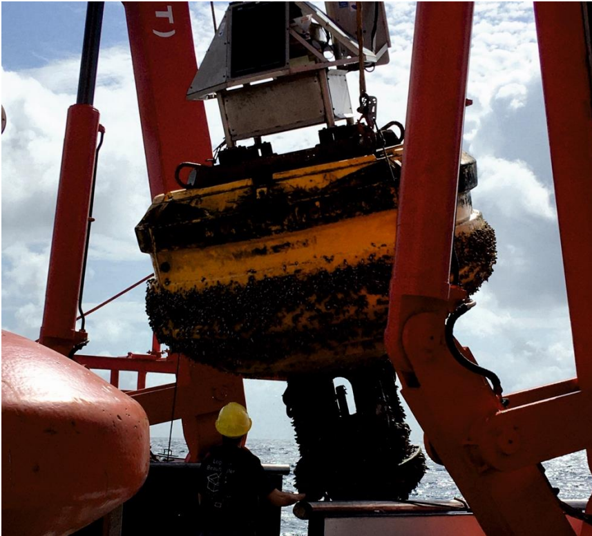
Picture 2. Recovery of dust buoy "Carmen" (Photo: Karin Zonneveld)
