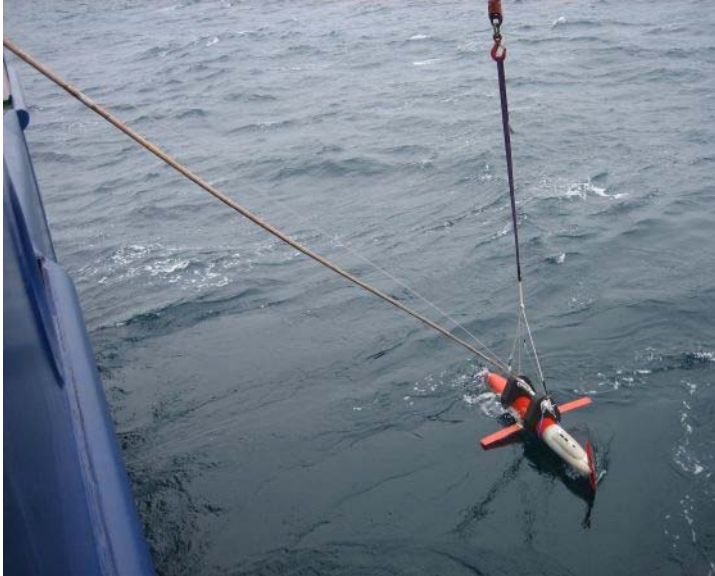
Spray 004 deployment: last verifications and mission launching (up left), crane lifting (up right), smooth immersion behind the ship (bottom left), and last “au revoir” (bottom right).
