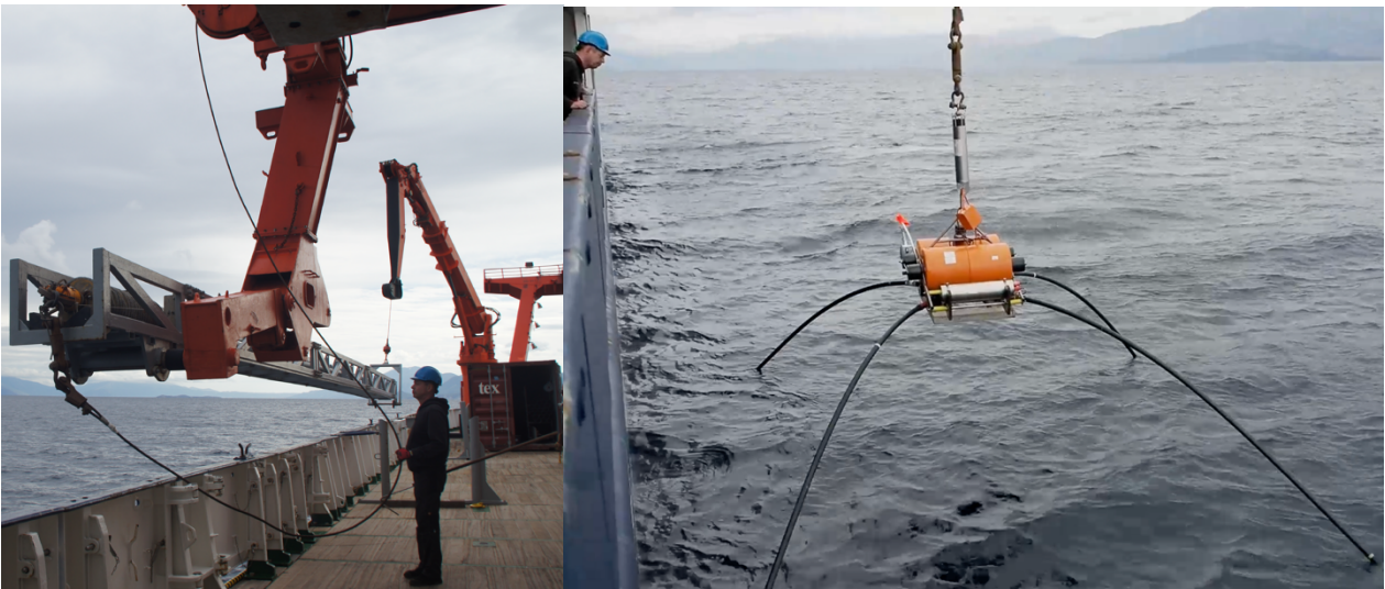
Deployment of gravity core (left) and OBEM (right).
