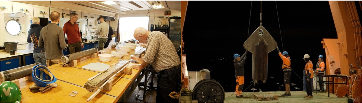
Analysis of gravity cores (left) and deployment of head of CSEM streamer (right)..
