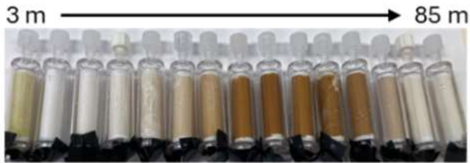
Figure 1: Mn oxide samples from Landsort Deep. Picture illustrates the particles collected on filters spanning the depth range from 3m to 85m. The brown color is indicative of Mn oxides. The peak of Mn oxide concentration is observed at 80m at the base of the chemocline.
