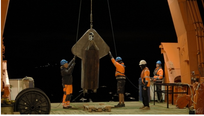
Deployment of electromagnetic transmitter.
