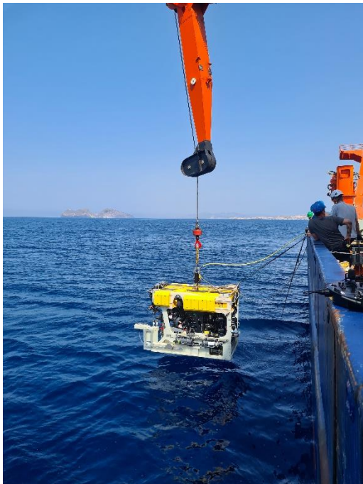
Figure 1 (left): The MARUM ROV -SQUID is lowered into the water (Photo: Solveig Bühring)
