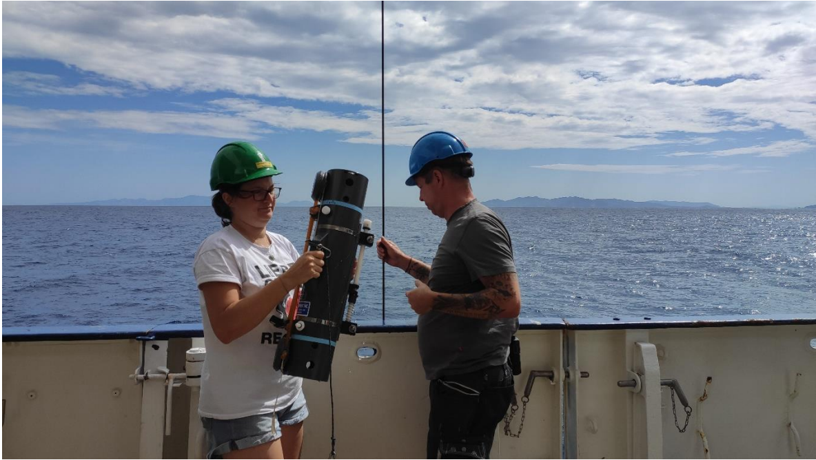
Figure 5: Eva Meckel (Constructor University) and boatman Michael Zeigert fix a trace-metal GoFlo bottle on a Kevlar rope (Photo: Andrea Koschinsky)
