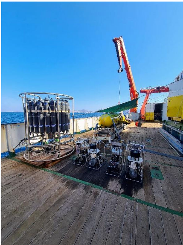
Figure 1: Main equipment this week: CTD water sampler rosette on the left, in-situ pumps on the right, and behind it the AUV MARUM-SEAL under its sun protection sail.
