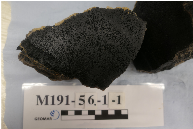
Fig.2: Moderately vesicular mafic lava with fresh olivine phenocrysts, suitable for all kinds of geochemical analyzes. The absence of secondary vesicle fillings greatly facilitates rock preparation at the home institutions. Photo: M. Felgendreher
