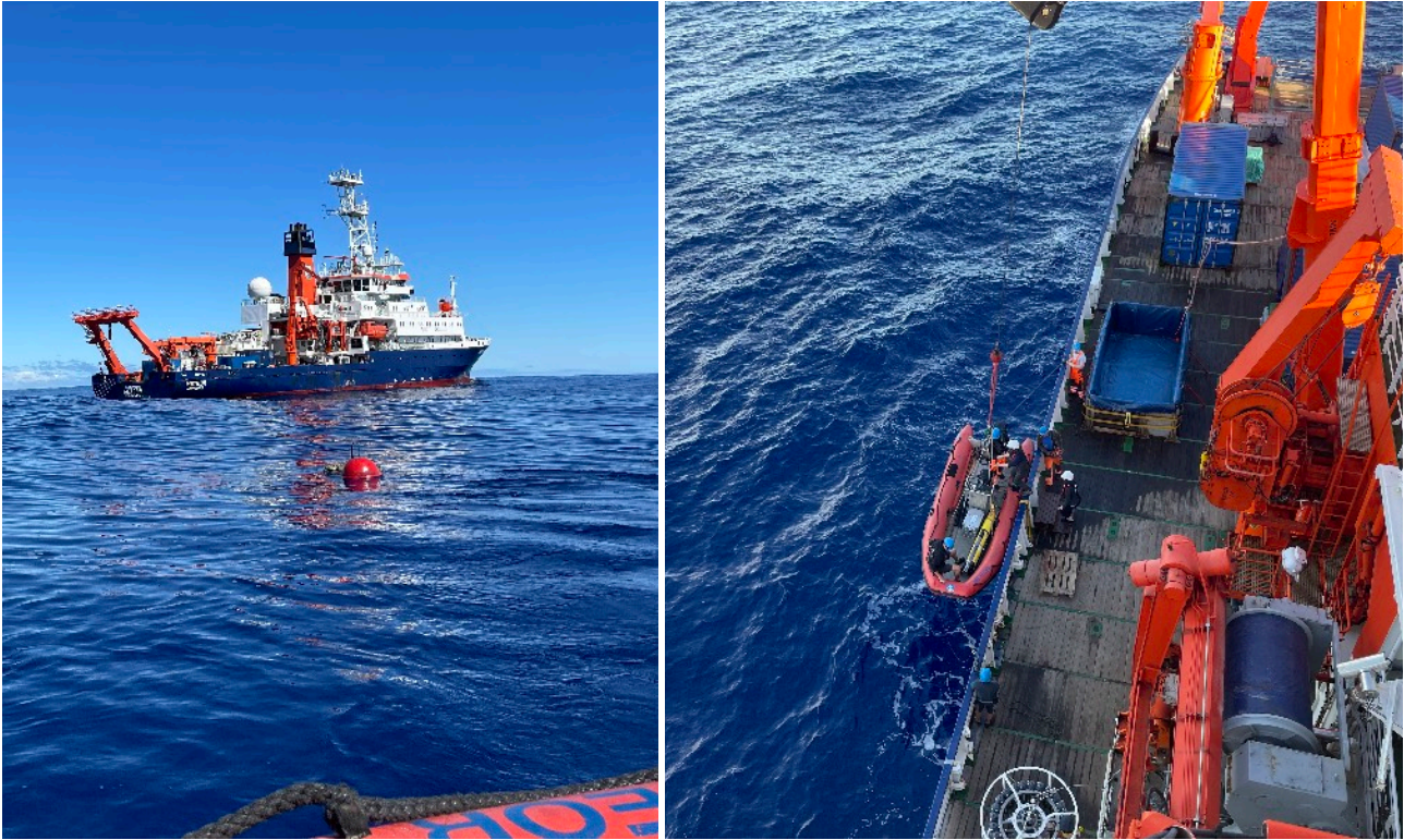
Fig. 2: Deployment of a surface drifter (left) and recovery a glider (right), both in ideal weather conditions from an inflatable boat (photos: L. Aschenbeck).
