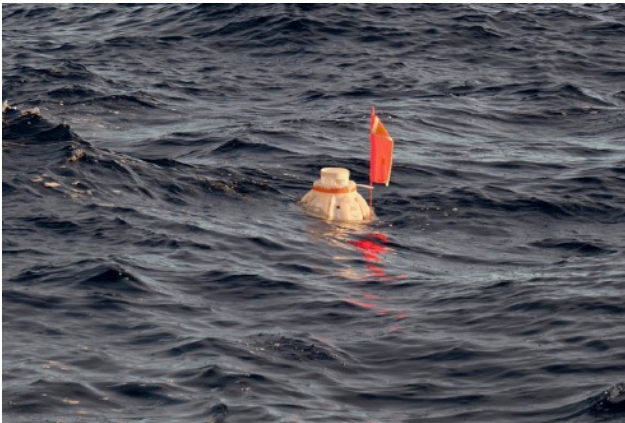
Fig. 2: Mooring recovery with an ADCP in a large buoyancy sphere (top left), and the acoustic releases with small buoyancy spheres (top right). Bottom: Recovery of an inverted echo sounder (PIES). All in the best weather conditions. (Photos: A. Welsch and C. Mertens).
