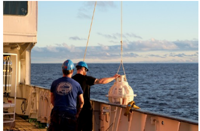
Fig. 2: Mooring recovery with an ADCP in a large buoyancy sphere (top left), and the acoustic releases with small buoyancy spheres (top right). Bottom: Recovery of an inverted echo sounder (PIES). All in the best weather conditions. (Photos: A. Welsch and C. Mertens).
